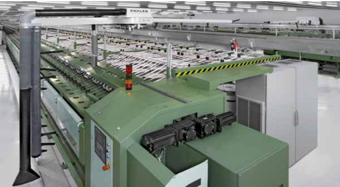
Modern travelling cleaners over speed frames guarantee a high degree of cleanliness by providing continuous blowing and suction to the drafting system, flyer zone and floor, and consequently create the best possible conditions for regular roving. Moreover, the waste from the drafting system cleaning devices can be collected by the cleaner.
