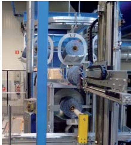
*These doff- and handling systems fit perfectly into the production area and environment. Several doffing unit types are available for the different winding machines. The equipment is so conceived that the production performance is granted with consideration of the operators.*
