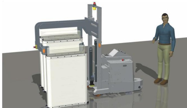
Automatic Guided Vehicle: Special designed gripper systems allow individual can positioning.
