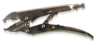
959.1302 Fitting pliers Carbon-fibre traverse rod SE 9 / 10 / SC / SQ
