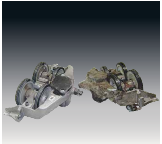
Comparison of bearing with ProFiL ® Cartridge (left) with oil-lubricated bearing (right) after 8 weeks of application spinning 100 % cotton, Ne 24 at 120,000 rpm on the same machine
